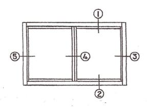
WINDOW CONFIGURATIONS: XX, XOX, OXO (OTHER CONFIGURATIONS AVAILABLE) **WINDOW ELEVATION** SCALE: 3" = 1'-0"
